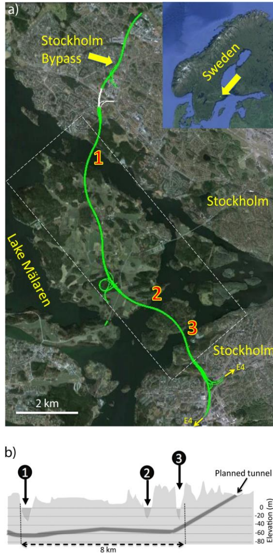
Figure 1. (a) The Stockholm Bypass project plan. The green line is the planned track, and the frame on the top-right corner shows the location of the study area in Sweden. (b) Cross section of part of the planned tunnels (marked with the dashed white box in panel [a]) below Lake Mälaren. Sites 1, 2, and 3 are where the case study was conducted (Figure is modified from Bastani et al. 2015).
